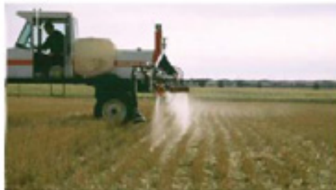
Figure 3. Air induction nozzles at 70 psi. (Wolf)
